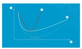
A = Losses B = Speed 1 = Total losses traditional element 2 = Total losses Atlas Copco element
